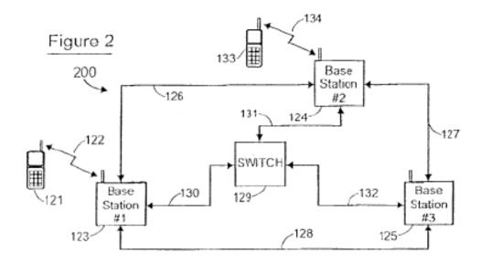
Pet. App. 80a (Figure 2). In this new architecture, the wireless communication protocol is divided into two parts, with certain protocol functionality (including functionality that is time-sensitive) performed at the base station and other functionality (including functionality that is not time-sensitive) performed at the switch. Pet. App. 138a-39a.
