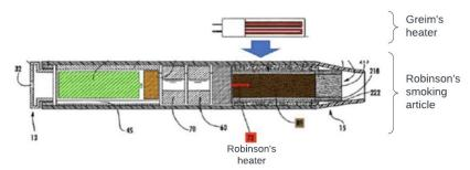
J.A. 160 (annotations added). The figure above shows Greim's heater alongside a cross-sectional view of Robinson's smoking article. Robinson's smoking article contains heating element 72 extending into the tobacco segment 89. See Robinson, col. 27 ll. 31–39, Fig. 3.
